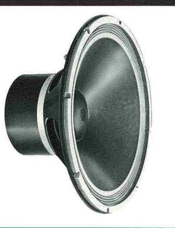
The ALTEC 515B is a 15-inch low-frequency loudspeaker with a frequency response trom 20 Hz to 1000 Hz. When used in conjunction with ALTEC 288C or 291-16A drivers, N-500C or N-500F dividing network and multicellular horn of the desired size and coverage angle, the 515B becomes an integral part of the identical ALTEC 'Voice of the Theatre'® loudspeaker system. These systems are currently installed in a majority of the largest and finest theatres, auditoriums and concert areas.
