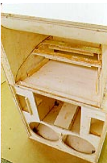
The shape of this horn flare has been cut by a CNC router. A 3mm sheet of birch ply will be inserted in the slot to form the flare, which is braced with wood formers. The cavity behind the flare will be filled with high density structural foam.
