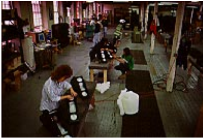
In the final assembly process, drivers and crossovers are installed in the painted enclosures.
