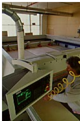
Computer-programmed saws cut pieces to exacting tolerances.
