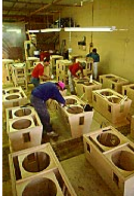
The modern adhesives that hold the cabinets together are stronger than wood screws, staples and even the wood itself.
