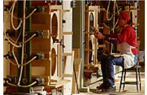
EAW loudspeaker enclosures are built using modern manufactured wood products designed for high density and tensile strength.
