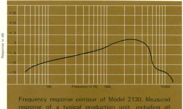
response of a typical production unit, including all peaks and dips, does not deviate more than 3 dB from the above curve.
