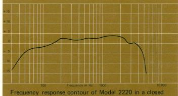
box of six cubic feet internal volume. Measured response of a typical production unit, including all peaks and dips, does not deviate more than 2 dB from the above curve. Additional acoustic loading (horn or ported enclosure) will further extend bass response.
