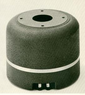
Model 2440 is the most massive professional quality compression driver in the industry. It has a four inch voice coil, and an Alnico magnetic structure weighing more than 25 pounds. It can take the most explosive transients in stride, and reproduce them at thunderous levels with flawless accuracy. Model 2440 is built to typical JBL standards of precision.
