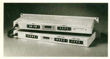
Input and output terminals for the 5231 and 5232 are as shown. The dual channels of the 5232 can be utilized for tri-amplifications of a single loudspeaker system by connecting the high frequency output of one channel to the input terminals of the other channel.
