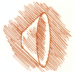
A speaker cone with the apex truncated
