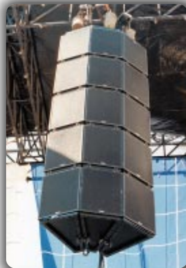
(Right) Each KF900 array used for Promise Keepers' 1997 events was assembled and flown by a crew of three in less than 30 minutes. (Left) Since the beams are focused vertically with DSP, KF900 arrays are always dead hung. This eliminates the need to aim the array physically.
