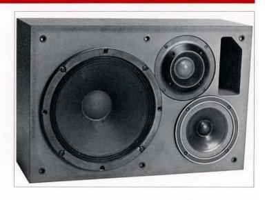
The low frequency section consists of an RCF L12/584 high efficiency driver mounted in a compact enclosure. The vent tuning is optimized for flat response and maximum output above 100 Hz. When used for all music reproduction applications, the DS123B is intended to work with a subwoofer system such as the EAW VB118 18 inch or VB215 dual 15 inch vented low frequency systems.
