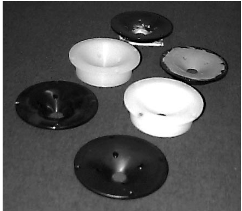
JF100 wave guide prototypes. Various forms are built up using nylon, fiberglass, and clay. Test data shows the results of modifications and refinements.
