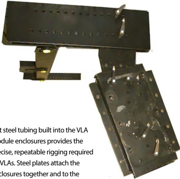
Flat steel tubing built into the VLA module enclosures provides the precise, repeatable rigging required by VLAs. Steel plates attach the enclosures together and to the specially designed fly bar. The added strength of steel allows arrays as large as 12 modules to be safely flown.
