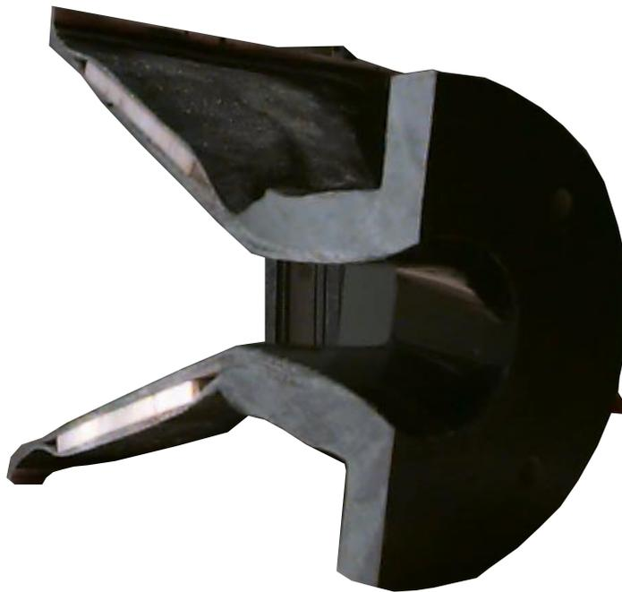
This cutaway view illustrates the “reverse draft” or “undercut” portion of the horn throat.
