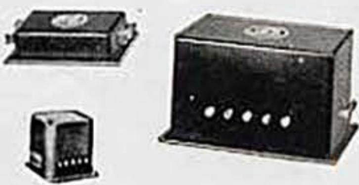
All EV Crossovers use high Q air core coils. Insertion loss less than 3 db, phase rotation 270° (135° in X-825-1) attenuation 12 db per octave in 3½ section, 6 db per octave in ½ section crossovers.
