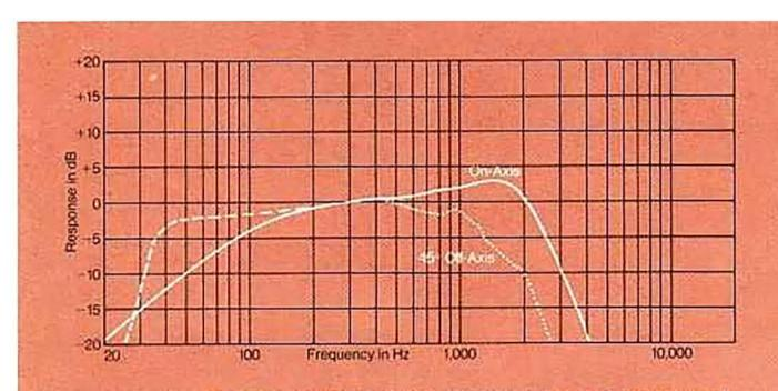
Frequency response contour of the 2225H/J taken in a hemispherical free-field environment, a closed box of 140 L (5 ft3) internal volume enclosing the rear of the driver. Measured response of a typical production unit, including all peaks and dips, does not deviate more than 2 dB from the above curve. The dashed curve represents the response from a 160 cm2 (25 in2) port with a 13 cm (5 in) long duct tuning this enclosure to 40 Hz.
