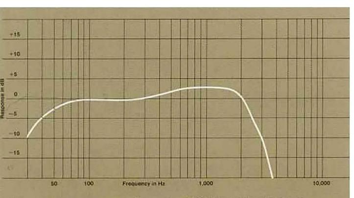
Frequency response contour of the 2231 in a closed box of 5 cubic feet (140 litres) internal volume. Measured response of a typical production unit, including all peaks and dips, does not deviate more than 2 dB from the above curve. Additional acoustic loading (passive radiator or port) will further extend bass response.
