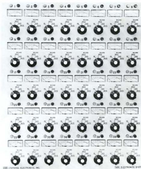
Front view of 40-track sync panel
