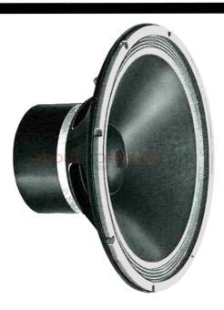
The ALTEC 515B is a 15-inch low-frequency loudspeaker with a frequency response trom 20 Hz to 1000 Hz. When used in conjunction with ALTEC 288C or 291-16A drivers, N-500C or N-500F dividing network and multicellular horn of the desired size and coverage angle, the 515B becomes an integral part of the identical ALTEC 'Voice of the Theatre'<sup>®</sup> loudspeaker system. These systems are currently installed in a majority of the largest and finest theatres, auditoriums and concert areas.
